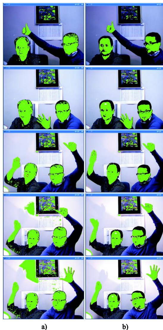
Figure 18. Results of the real-time segmentations with different illumination levels: (a) segmentation of original images captured directly from the camera, (b) segmentation of the images after the colour injection.
