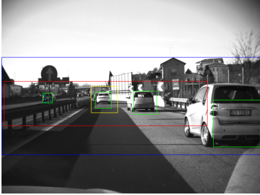
Fig. 3. [Best viewed in color] Example of the three vehicle detection stages working. Green boxes represent detections, blue the near-window, red the far-window, yellow the intermediate window (vehicle-specific) and the points depicted in blue in the vehicle of the left represent Optical Flow.
