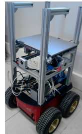
Fig. 6. Autonomous robot Pioneer 3-AT with 4 cameras mounted on a metallic structure.
