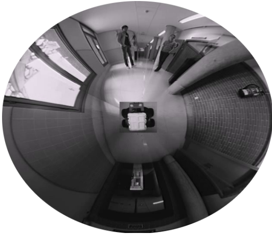
Fig. 8. Circular view representation of the robot surroundings after warping and blending of the 4 images.
