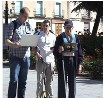
Fig. 6. The stereo camera system is attached to chest of the visually impaired user by means of a non-invasive orthopedic vest. Then the camera is connected to a small laptop by means of a firewire cable.
