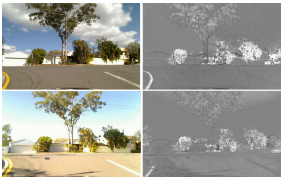
Fig. 3. An example of illumination invariance application in the St Lucia dataset between two places at different hours. The images on right are the illumination invariant transformation of the left images. It can be seen how this approach reduces the effects produced by sunlight and shadows.
